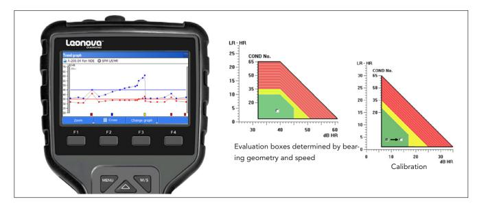
The LR/HR method was developed from the original Shock Pulse Method for condition diagnosis of rolling element bearings. It allows a precision analysis of oil film condition in the rolling interface and contains computation models for finding the optimal lubricant. Poor lubrication is the root cause of most bearing failures.
