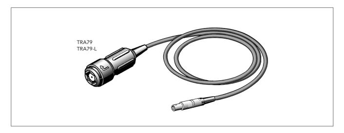
TRA79 is a shock pulse transducer with quick connector, used together with the handheld instrument Leonova Diamond® and Emerald®, for measurements on permanently installed adapters. The quick connector forms a bayonet connection together with the permanently installed adapter. Standard cable length is 1.5 m. Other lengths up to 20 m can be ordered.
