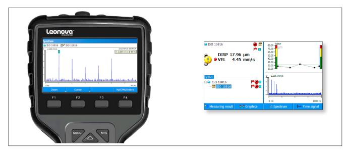
Broadband vibration measurement is the most widely used and cost-efficient method for the diagnosis of general machine condition.
