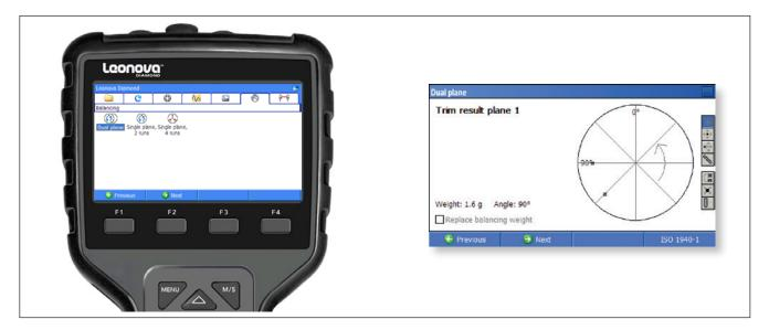
Single and dual plane balancing are optional Leonova functions for either limited or unlimited use. In case of limited use, credits are deducted for each vibration measurement.
