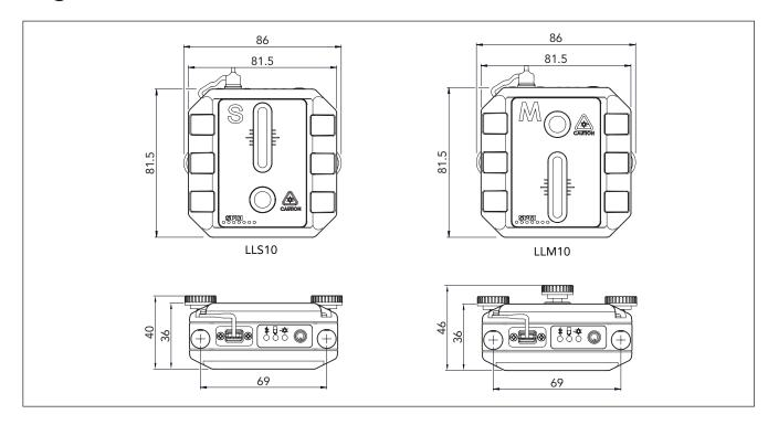
The alignment sensors LLS10 and LLM10 are two measuring units for shaft alignment with the multi-function datalogger Leonova Diamond. The alignment sensors are identical with exception of the position of laser detector and the knob for adjustment of the laser on the alignment sensor marked M. The alignment sensors communicate wirelessly with Leonova Diamond via Bluetooth. The Bluetooth dongle LLD10 for Leonova Diamond is included in LineLazer Alignment Kit LLA450 and LLA451.
