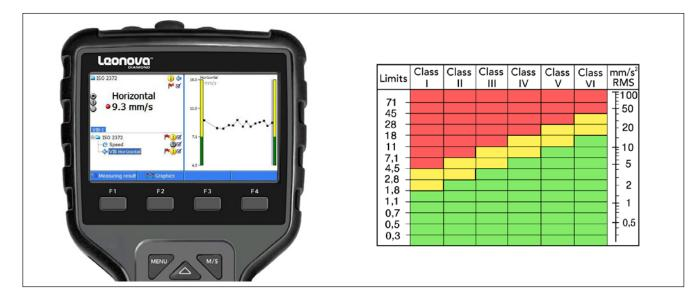
Broadband vibration measurement is the most widely used and cost-efficient method for the diagnosis of general machine condition. There are two ISO recommendations concerning this type of machine condition monitoring; the much used ISO 2372 and the more recent ISO 10816, which is a ongoing replacement of the older standard.
