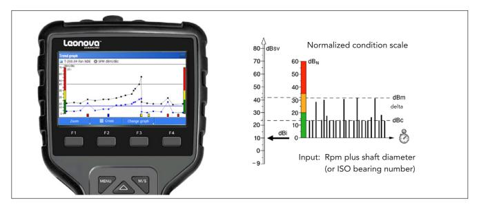
For over 40 years, the original Shock Pulse Method (SPM) has been very successfully used to obtain a fast, easy and reliable diagnosis of the operating condition of rolling element bearings.
