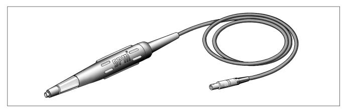
TRA78 is a handheld probe, used together with Leonova Diamond® and Emerald®. The probe is directionally sensitive and must be held aligned against the bearing and not deviate from this direction by more than  $\pm 5^\circ$ . The probe tip is spring loaded and moves within a sleeve made of chloroprene rubber (neoprene) and tolerates 110 °C (230 °F). Standard cable length is 1.5 m. Other lengths up to 20 m can be ordered.
