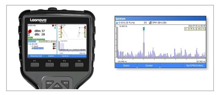
The purpose of SPM Spectrum is to verify the source of high shock pulse readings. Shocks generated by damaged bearings will typically have an occurrence pattern matching the ball pass frequency over the rotating race. Shocks from e. g. damaged gears have different patterns, while random shocks from disturbance sources have none.
