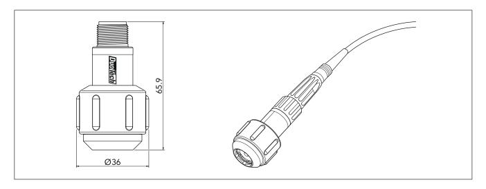
TRC150 is a DuoTech accelerometer with quick connector, used together with the handheld instrument Leonova Diamond and Emerald, for measurements on permanently installed adapters. The quick connector forms a bayonet connection together with the permanently installed adapter. The accelerometer is internally isolated in a Faraday shield providing maximum protection from ground loops and RF interference.
