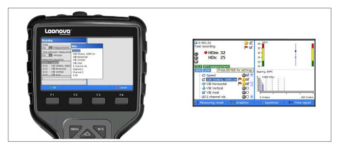
The Recording function is part of the platform, always included for unlimited use. It allows the user to measure and record measuring results over longer periods of time. The recording function is an analysis tool which can show the interaction of various condition parameters over time.
