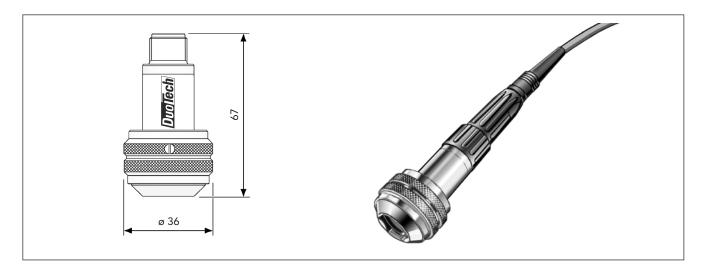
TRC100 is a DuoTech accelerometer with quick connector, used together with the handheld instrument Leonova Diamond and Emerald, for measurements on permanently installed adapters. The quick connector forms a bayonet connection together with the permanently installed adapter. The accelerometer is internally isolated in a Faraday shield providing maximum protection from ground loops and RF interference.
