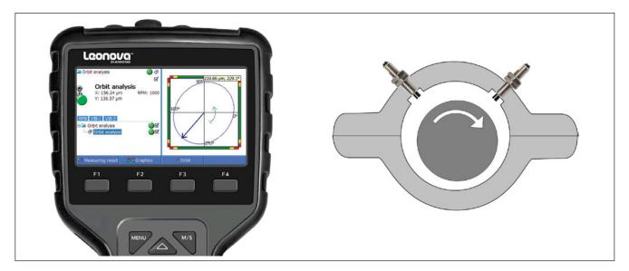
Orbit analysis and Shaft centerline plot is a vibration measurement function offered with Leonova Diamond®, for either unlimited (DIA138) or limited use (DIA238). The resulting orbit graph shows the movement of the shaft's centerline and is used to detect failures like rubs, unbalance, misalignment or oil whip on machinery with journal bearings.
