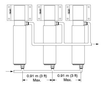
Figure 6 Parallel Installation
