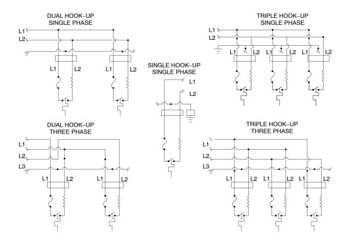
Figure 4 NH-4 Heater Wiring Diagrams
