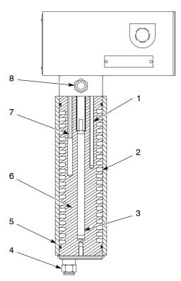
Figure 2 Cutaway View of Heater Components
