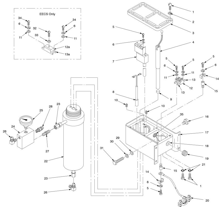
Figure 13 Stainless Steel NH-4 Heaters – Single and Twin Passage, 115, 230, 230 EECS, 460 Volt
