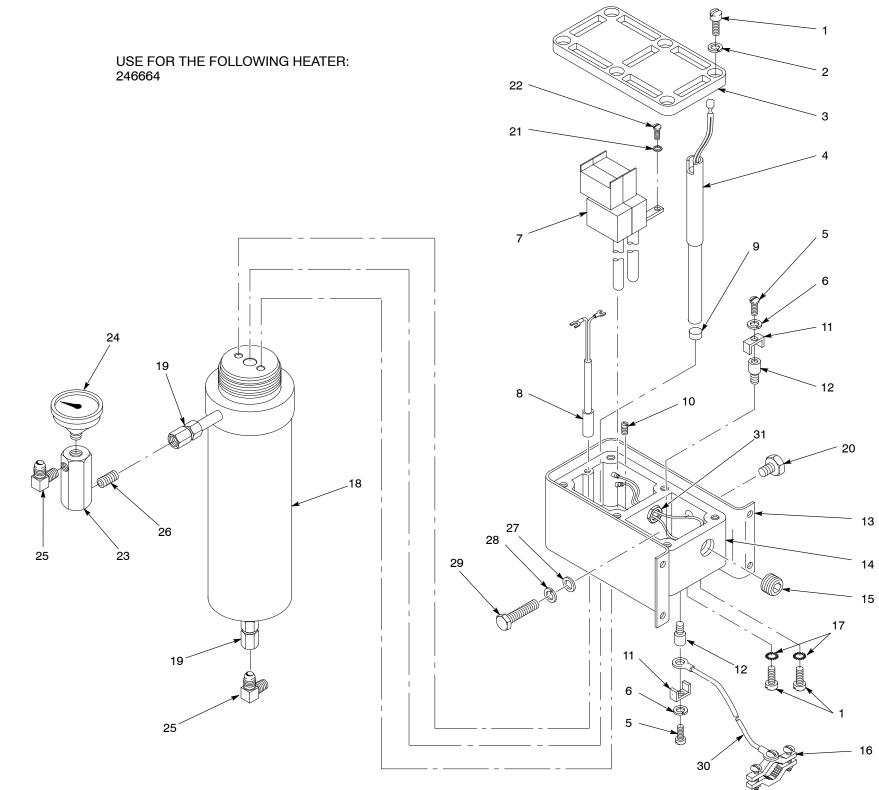
Figure 14 Stainless Steel NH-4 Heaters – Single and Twin Passage, 200 Volt – Japan Only
