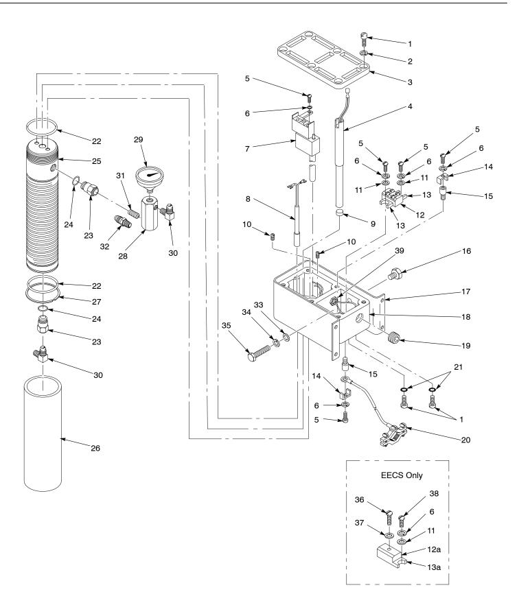
Figure 12 Standard Steel Plated NH-4 Heaters – Single and Twin Passage, 230, 240, 380, 460 Volt
