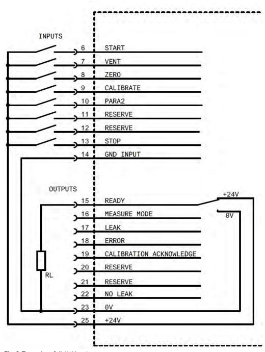
Fig. 9: Examples of digital inputs
