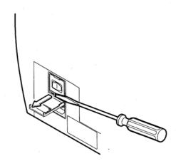
Fig. 19: Removing fuses
