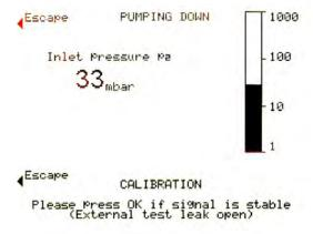
During a calibration with an external calibration leak or an internal calibration leak in the "Manual internal" mode, the stability of the signal must be confirmed using the "OK" button.
