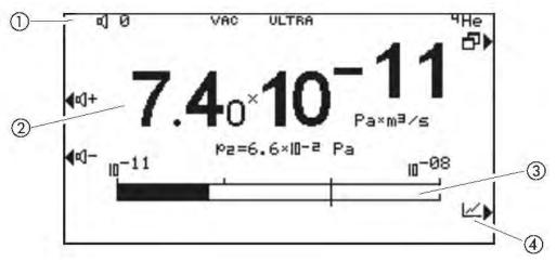
Fig. 5: Numerical display, measuring screen
