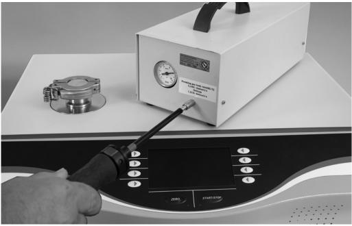
Fig. 17: Sniff test on an external calibration leak
