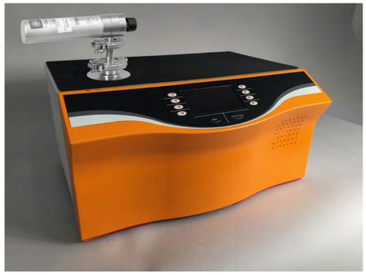
Fig. 15: Checking an external calibration leak
