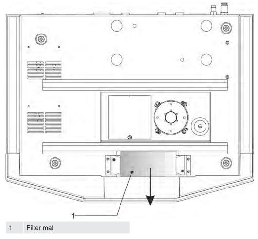
Depending on the operating conditions, the recommended inspection interval for the filter mat varies between weekly and annually. The filter plate for fan 1 can be reached from the front of the device and replaced without tools.
