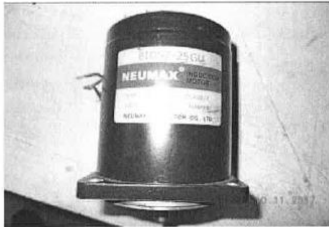
A/E J.C.W Temperature control valve Induction Motor NEUMAX ACTUATOR CO., LTD 8 IDS 2-25 GU 25W, 220V, 50Hz, F-Class, 0.57A, 4 uF, 1250rpm
