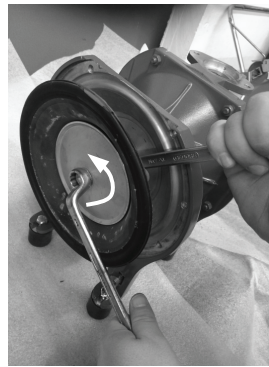
Pic. 4: Diaphragm disassembly
