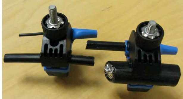
Picture 2: Samples after the test with conductor configuration min-min and max-max
