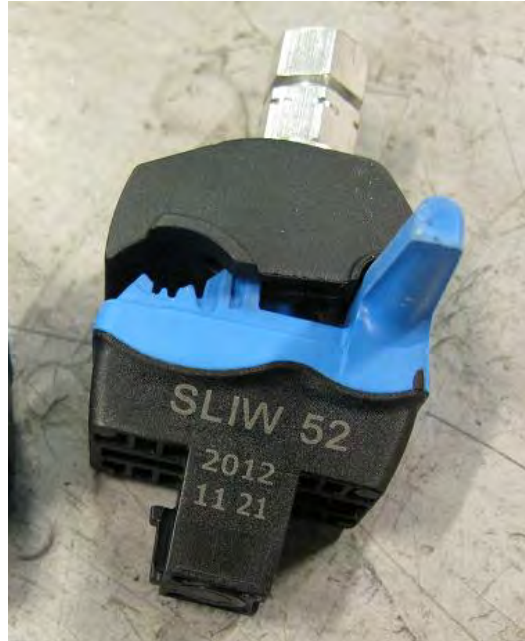
Picture 2: Connector after the test
