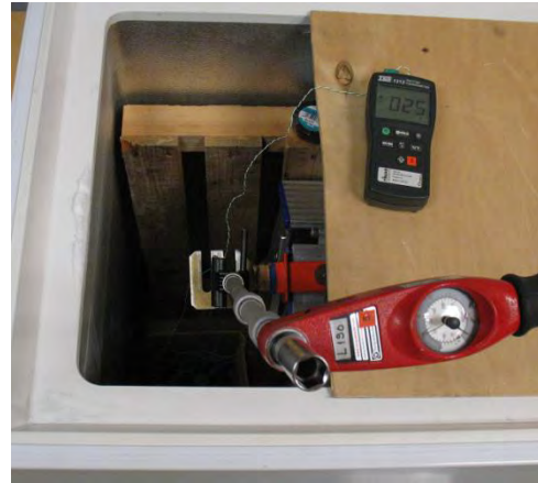
Pictures 3 and 4: Test in 50 °C oven and in -25 °C freezer
