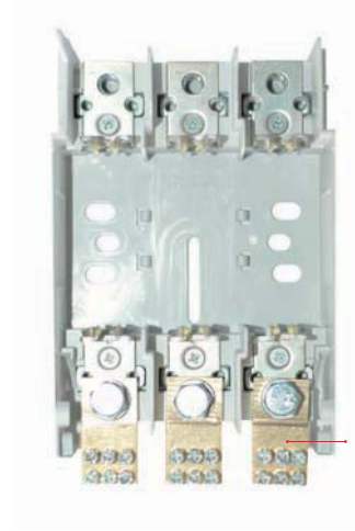
RBK 00-W with terminal clamp 1x16 mm 2 , 2x25 mm 2 (view of fuse switch disconnector without fuse-link cover and terminal shrouds)
