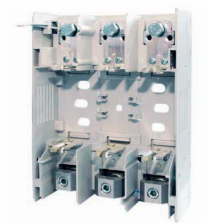
RBK 1 VD-M for installation on mounting plate, picture of fuse switch disconnecter without fuse links cover and terminal shrouds, top cable terminal - M screws, bottom cable terminal - V-clamps, (RBK 1 VG-M - bottom cable terminal - M screws, top cable terminal - V-clamps)
