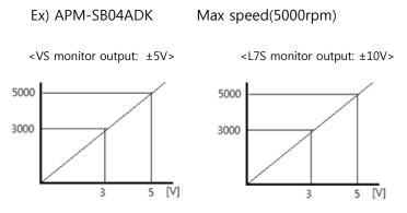
\* L7S : To enter same output voltage as VS, Set DAC output sale value '1000' in P0-23
