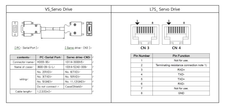
Note) The TXD and RXD in the above table are based on the servo drive. Please refer to Manual Chapter 4 for detail information
