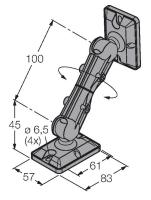
7030296 Arm bracket for UHF RFID read/write heads TNxxx-Q175L200-H1147, TNxxx-Q240L280-H1147 and TNxxx-Q280L640-H1147
