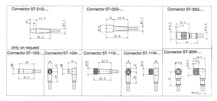
Part-Number of cables which correspond to the Meto-Fer connector 01 and 02 (cable cross section: 0.14mm\_)
