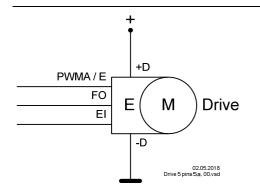
E stands for integrated electronics. M stands for motor. Drive stands for motor with axial integrated electronics.
