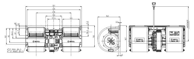
Fixing recommendation: use M4 bolts for fixing. Nominal tightening torque 3 +1/0 Nm Nominal torque defined for brand new, clean and lubricant-free bolts.
