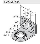
3072587 Mounting bracket, steel, blackfinished, for EZ-ARRAY and EZ-SCREEN standard 14 & 30 mm
