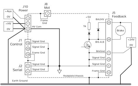
Earthing connections for power supplies should be as close as possible to elimimate potential differences between power supply OV terminals.
